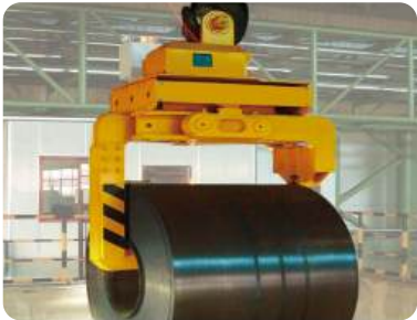
Coil Lifting Tong Vertical coil lifts
