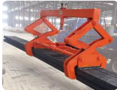
Billets Handling Clamp Hot billet transfer
