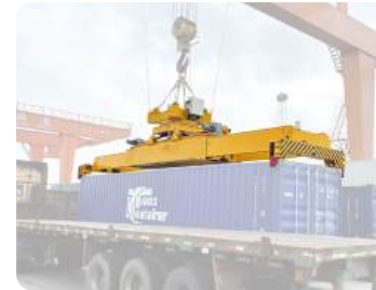
Container Spreader 20/40/45-ft ISO containers
