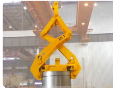
Coil Lifter Slit coil packages
