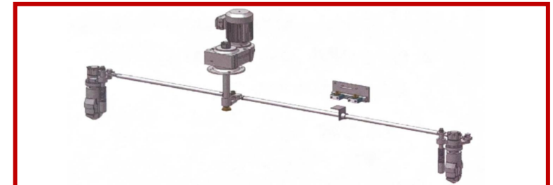
Electric Spreader End Twistlock Mechanism
